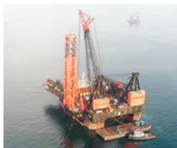
**Sound-proof encasing/protection** The offshore industry pays little attention to the relatively high sound levels in pumping areas, engine spaces and areas such as the shaker house and doghouse. Discom designs, manufactures and installs sound-proof facilities in order to protect the environment and staff from these sound sources. That is how the living conditions onboard of these installations have improved significantly.
